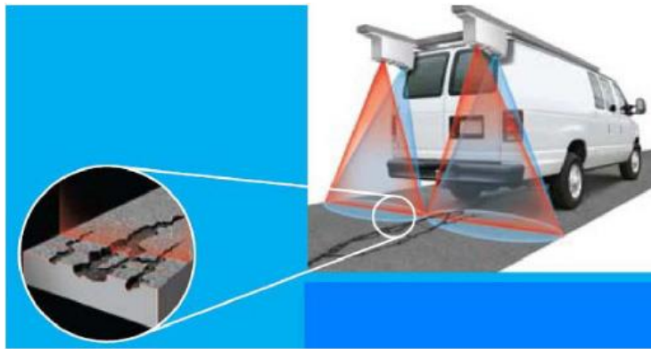
Figura 6 - Sistema LCMS (Laser crack measurement system)
